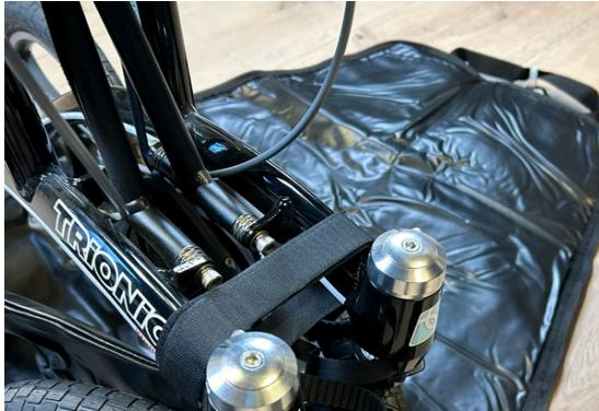
④ Secure the folded frame with the integrated Velcro strap.
