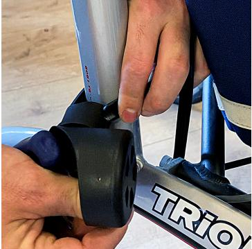
④ Attach the lower holder to the frame
