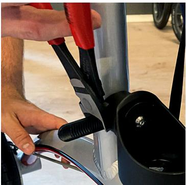
⑥ Cut the excessive length of the strap
