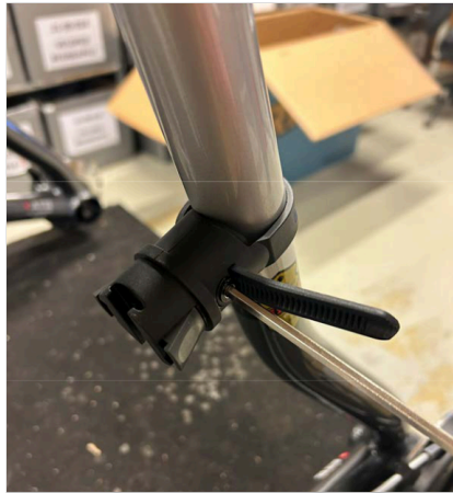
⑥ Tighten the screw/strap with the 4 mm allen key until the strap is tight.
