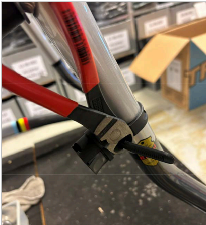
⑦ Cut off the excessive length of the strap with a cable cutter or knife.
