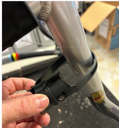
④ Wrap the strap around the Veloped rear vertical frame tube (on the Walker, the semi-vertical frame tube).
