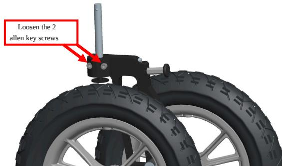
1. Loosen the 2 allen-key screws, and push the QR-axle down through the fork until the big axle nut is visible.
