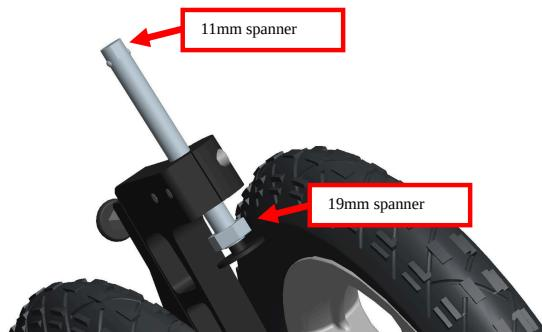
2. Adjust the length of the QR-axle with 11 mm and 19 mm spanners. Keep the QR-axle from rotating by holding it at its end with the 11 mm spanner. Adjust the nut with the 19 mm spanner. If the axle doesn't lock into the frame, screwing the nut  $\frac{1}{4}$ - $\frac{1}{2}$  a turn anti-clockwise is sufficient.
